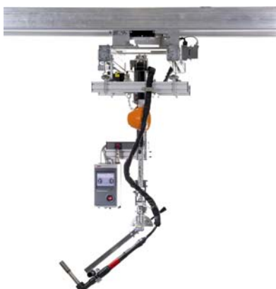
iTeleskop pivoted with SMX30 nutrunner control and HCX2 handheld nutrunner
